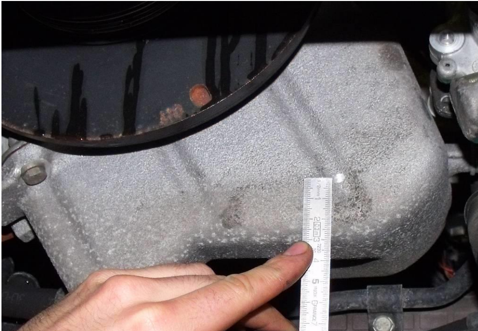
Illustration 8: Position of the oil return flange
