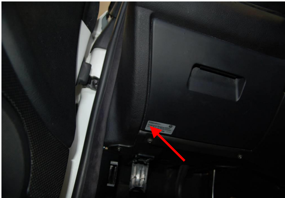
Illustration 38: Sticker ECU at OBD socket
